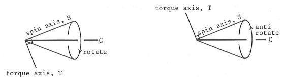
Let S denote the spin axis, and C the axis of the cone. If you try and rotate S around C in the same direction as the spin you will in fact be applying a torque whose axis T is at right-angles to S and points inwards towards C. By the gyro law S will move towards T, and appear to be attracted towards C, thereby helping you to rotate it around the cone.
