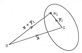
Therefore the acceleration of  $m_i$  is  $\ddot{x} + \ddot{y}_i$ , by Lemma 3. Let  $\mathbf{F}_{ij}$  be the internal force on  $m_i$  exerted by  $m_j$ . Apply Newton's law of linear motion to  $m_i$ :
