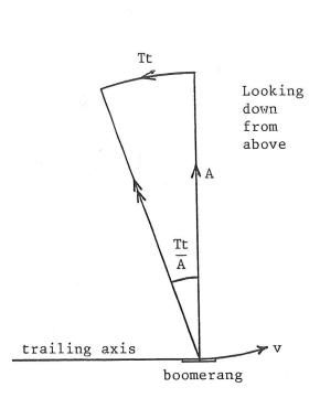
Therefore  $\Omega_1$  =  $\Omega_2$ , as required, and so the boomerang steers itself round the circle at exactly the right rate.
