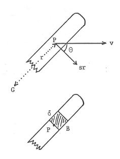
The significance of the aerodynamic factor is that it is a constant, depending only upon the aerodynamic shape of the blade, that enables one to calculate the lift generated by that blade according to the formula:
