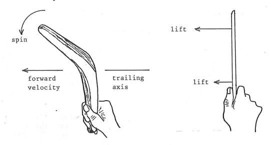
If you are right-handed hold the boomerang with the curved surface next to your face, so the lift will be to the left and the boomerang will fly in a circle to the left. A left-handed thrower needs a left-handed boomerang in which everything is reversed.
