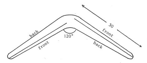
Use plywood about 6 mm thick. Each blade should be about 30 cm long and about 4-5 cm wide, and the angle between the blades about 120°. Use the same method of marking and shaping the blades, except that with plywood it is quicker to use a spokeshave to do most of the shaping and just use sandpaper for the final smooth finishing.
