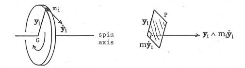
Each particle  $m_i$  at  $\boldsymbol{y}_i$  on the rim will have velocity  $\dot{\boldsymbol{y}}_i$  at right-angles to  $\boldsymbol{y}_i$ , and speed  $2\pi rs$ . Therefore
