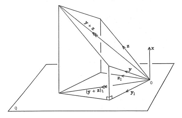
Firstly the parallelogram with sides  $\mathbf{y}$ ,  $\mathbf{z}$  is projected onto a second parallelogram with sides  $\mathbf{y_1}$ ,  $\mathbf{z_1}$  and
