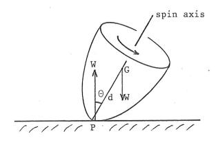
Ignoring friction, there are two forces acting on the top, the weight W downwards at the centre of gravity G and an equal and opposite upthrust at the point P in contact with the table. Since the forces are equal and opposite G remains stationary (for a proof see Appendix 1 Example 3). Let d be the distance from G to the tip. Show that the torque = Wdsin $\theta$ , approximately (only approximately because P is not quite at the tip).
