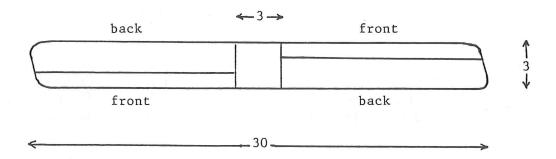
The front of each blade is identified by imagining rotating the piece anti-clockwise if you are right-handed, and clockwise if you are left-handed. The diagram is for a right-handed boomerang. Draw a line along each blade one third from the front. Sandpaper the top of each blade until it has cross-section like an aeroplane wing, rounded at the front, thickest where you drew the line, and streamlined at the back.
