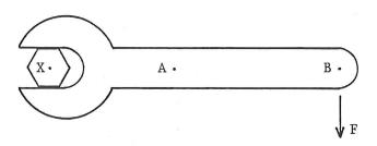
If you push down at B with force F what is the torque about X? The torque axis is perpendicular to the page; use the right-hand screw rule to determine the direction of the torque axis, whether it is towards you or away from you.
