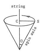
Let S be a point on the spin axis, and let C be the point on the string at the same height as S . By the gyro law S begins to move horizontally away from you at right-angles to CS . Therefore S precesses in the horizontal circle centre C . Therefore the spin axis precesses in a cone at constant angle  $\theta$  to the vertical.
