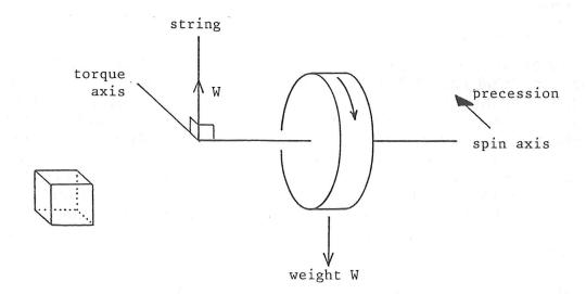
The two forces acting on the wheel are the weight W downwards and the equal and opposite pull upwards of the string. To work out the direction of the torque axis first identify the plane containing the two forces, which is the plane of the paper; then take a line perpendicular to the paper in the direction given by the right-hand screw rule, which is away from you. (This is indicated in the diagram by a line drawn parallel to an edge of the little cube in perspective.)
