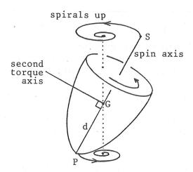
Verify that the second torque axis is in the plane of the paper perpendicular to the spin axis (approximately), and in the upwards direction. Deduce by the gyro law that the spin axis will rise, at the same time as precessing, and hence will spiral towards the vertical. When the spin axis becomes vertical it is called a *sleeping* top.
