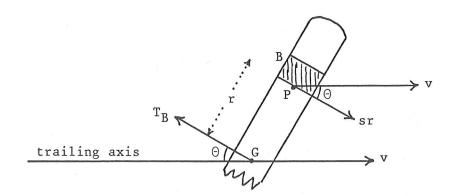
Show that the lift generated by B causes a torque  $T_{\rm B}$  about G in the direction shown in the diagram, and given by
