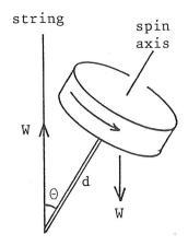
Show that the torque  $T=T_0sin\theta$ , where  $T_0$  denotes the torque when the spin axis is horizontal. What is the direction of the torque axis? Deduce that the spin axis precesses in a cone at a constant angle  $\theta$  to the vertical.
