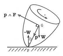
Let  ${\boldsymbol p}$  denote the vector GP, and  ${\boldsymbol \theta}$  the angle between  ${\boldsymbol p}$  and the vertical. The total torque  ${\boldsymbol T}$  about G is given by
