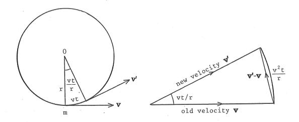
Therefore the vector  ${\bf v'}{\text -}{\bf v}$  is approximated by a circular arc of length  $v^2t/r$ , and is approximately parallel to mO. Therefore
